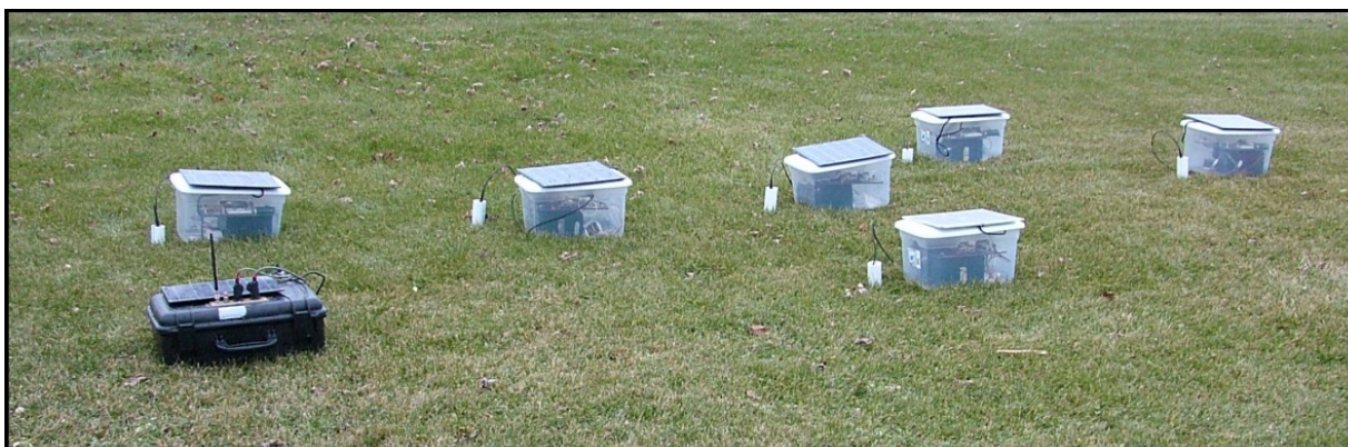
Figure 32 Experimental setup. Only the antennas were installed below the surface of the ground at a depth of 80 cm. The antennas were lowered into PVC tubes driven into the ground. Nodes were sealed from the elements inside of plastic containers. CS616 soil moisture probes monitored soil conditions between links. Data consisted of RSSI and soil moisture between all links. All data was routed and stored at the base station that consisted of custom data logger designed for this experiment.
