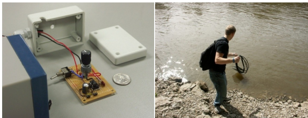
Figure 12 Left: Electronics and enclosure used for making conductivity measurements in freshwater. Right: Nick Sitter deploying the conductivity sensor into the Iowa River by the Stanley Hydraulic Laboratory in Iowa City.
