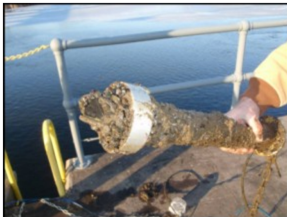
Figure 14 Example of bio-fouling of a sensor left in an underwater environment to collect data on water conditions.
